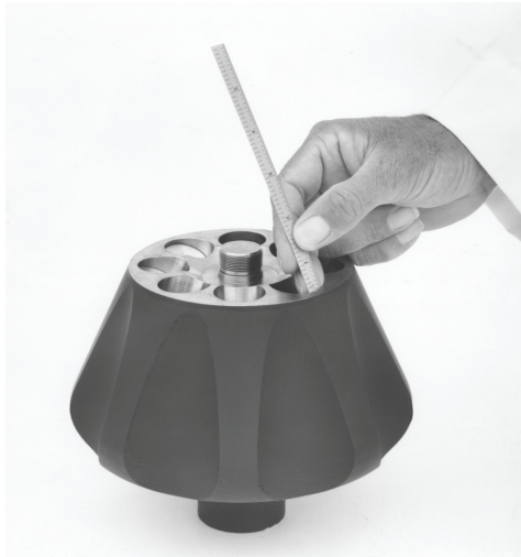
Figure 3 Measuring Distance from Cap to Rotor Tray
